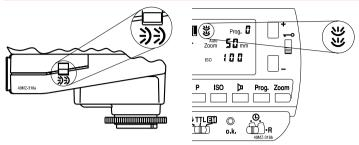
Fig. 16: Switching on the secondary reflector - Display
